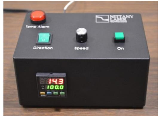
The cover window monitor displays the temperature of the cover window and warns the operator if the temperature rises indicating damage to the cover window.
