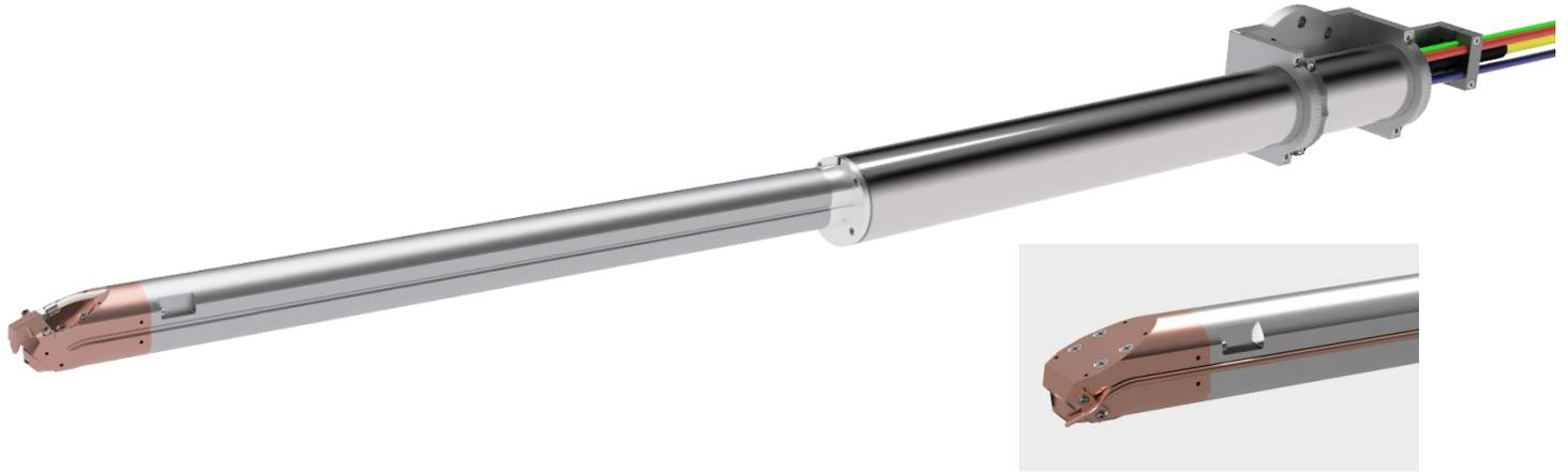
The 2” head is a highly reliable, robust tool for cladding with powder in bores as small as 2” in diameter and up to 24” deep. Switching between heads is accomplished by disconnecting the powder line, blowing the water out of the coolant lines, and removing the four mounting screws. The powder line is attached to the new head, and the four mounting screws secure the head to the base assembly. It is as simple as that!
