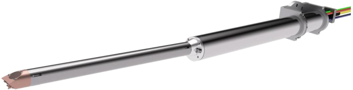
The 1.5” head is the smallest attachment currently available with the DB-IHS system. It is capable of cladding bores as small as 1.5” in diameter and up to 18” deep. As with all of our tools, the 1.5” head is a robust tool which used in production industrial settings around the world.
